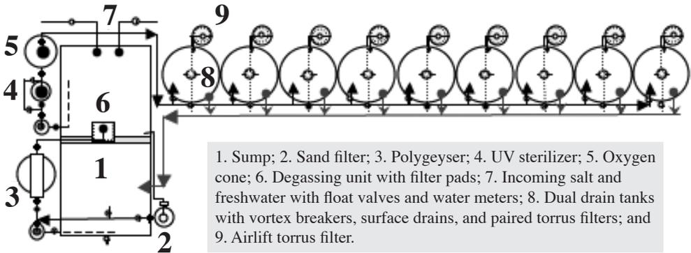
Figure 2. The low-energy hybrid recirculating aquaculture system design for Phase I to II (25 to 60 mm) juvenile red drum production. An airlift moves water between the tank and paired moving bed biofilter.
