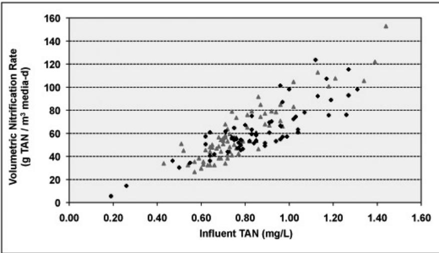
Figure 8. Volumetric nitrification rate (VTR) for a long flow pathway moving bed biofilter with 4.5 m<sup>3</sup> of MB<sup>3</sup> floating plastic media at varying TAN influent concentrations that was utilized in a low-head recirculating aquaculture system for Phase II to III (60 to > 180 mm) red drum fingerling production. Gray triangles represent the VTRs for System A biofilter and black diamonds represent the VTRs for System D biofilter.
