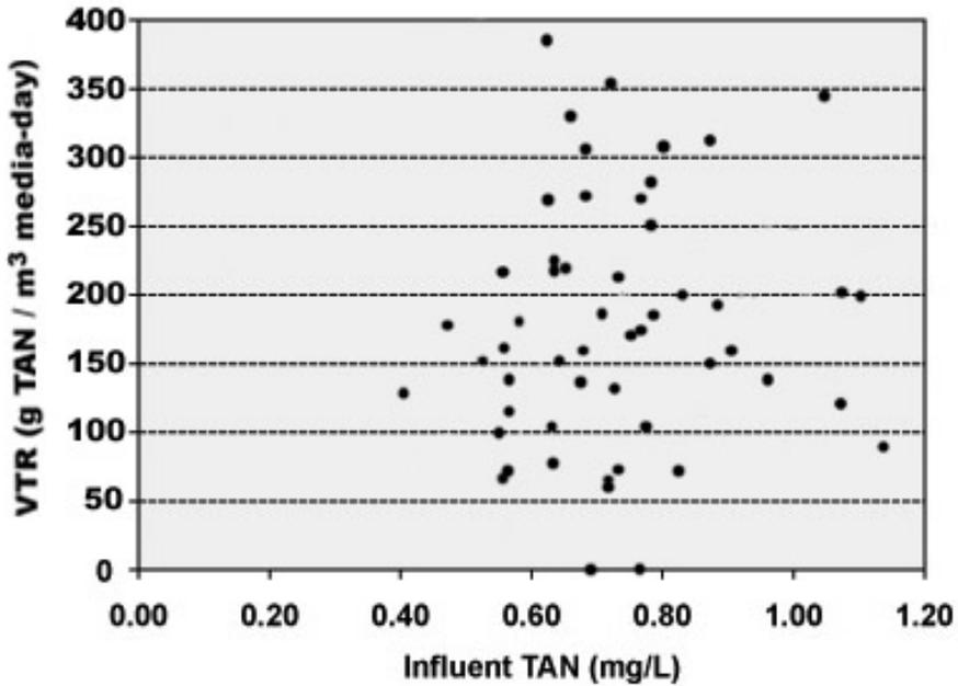
Figure 6. Volumetric nitrification rate (VTR) for a polygeyser filter with 0.11 m<sup>3</sup> of crimped floating plastic media utilized in the low-energy hybrid recirculating aquaculture system for Phase I to II (25 to 60 mm) red drum fingerling production. (N=56)
