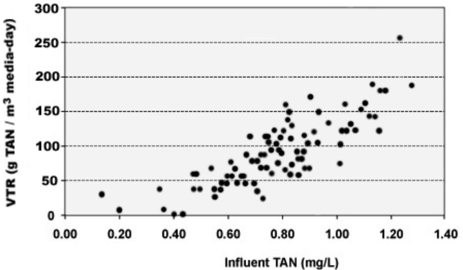
Figure 4. Volumetric nitrification rate (VTR) for a polygyser filter with 0.57 m<sup>3</sup> of EN media utilized in the low-head recirculating aquaculture system for Phase I to Phase II (25 to 60 mm) red drum fingerling production. (N=94)
