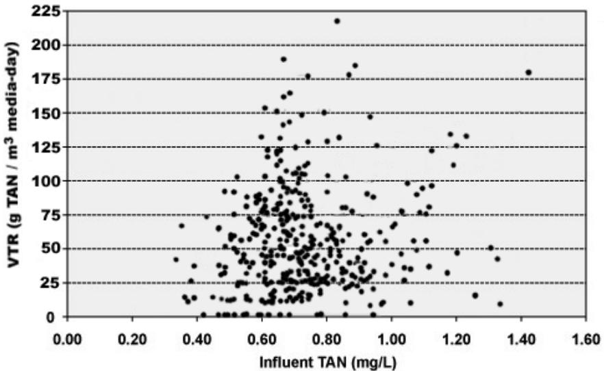
Figure 7. Volumetric nitrification rate (VTR) for the moving bed torrus filters with 0.11 m<sup>3</sup> of Kaldness media utilized in the low-energy hybrid recirculating aquaculture system for (Phase I to II mm) red drum fingerling production. (N=419)
