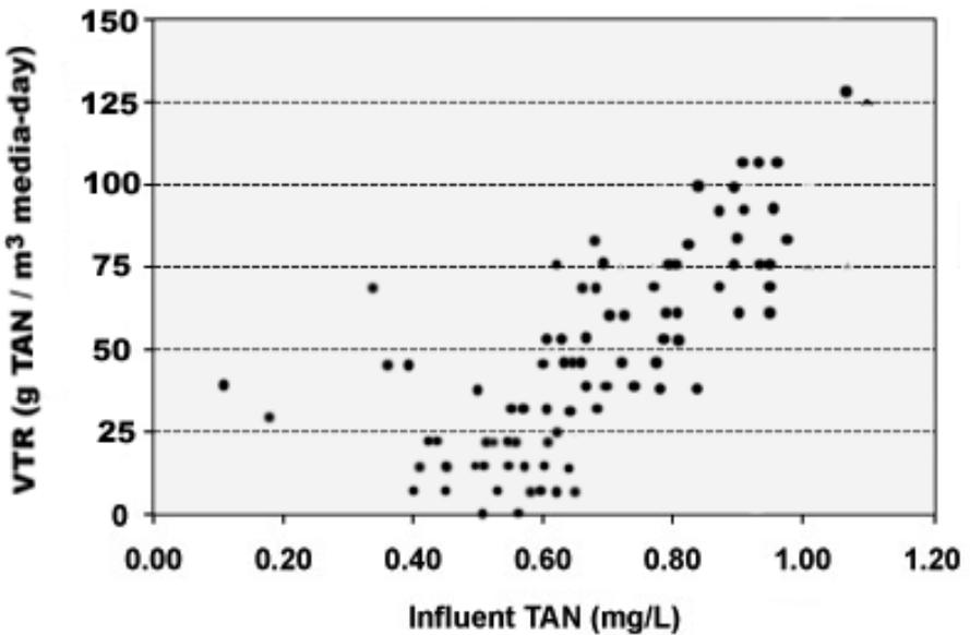
Figure 5. Volumetric nitrification rate (VTR) for a moving bead biofilter with 0.71 m<sup>3</sup> of floating plastic Kaldness K1 media utilized in the low-head recirculating aquaculture system for Phase I to II (25 to 60 mm) red drum fingerling production. (N=94)
