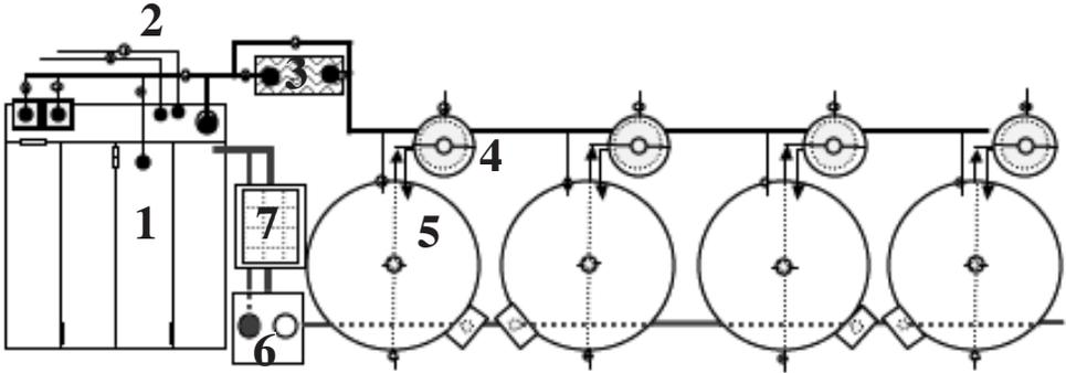
1. Long flow pathway moving bed reactor with cross-flow oxygenator, float valves, and propeller pump; 2. Incoming salt and freshwater lines with float valves and water meters; 3. UV sterilizer; 4. Torrus filters with 0.37 m<sup>3</sup> of MB<sup>3</sup> floating plastic media; 5. Three meter diameter tanks w/ center sump and sidebox drain; 6. Diverter box; and 7. Sixty micron screen rotary drum filter.
